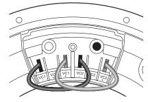
**Diagram B:** Parallel Connection (2 $\Omega$ ): Use two jumpers one from "VC1-" to "VC
