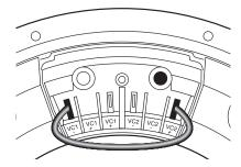
**Diagram A:** Series Connection (8 $\Omega$ ): Use one jumper from "VC1-" to "VC2+"
